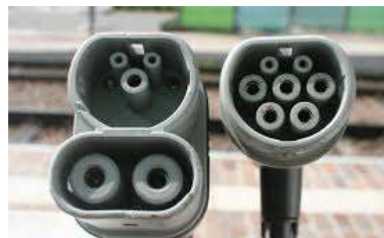
Figure 27 CCS Charge Port (left) and J1772 Charge Port (right)
