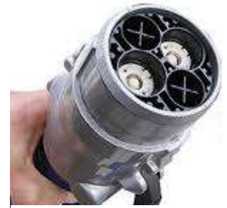
Figure 28 CHAdeMO Charge Port
