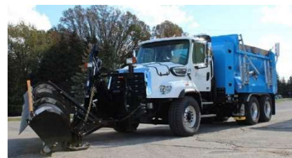
Figure 20 Freightliner 114SD CNG Truck Snow Plow in Oxford County
