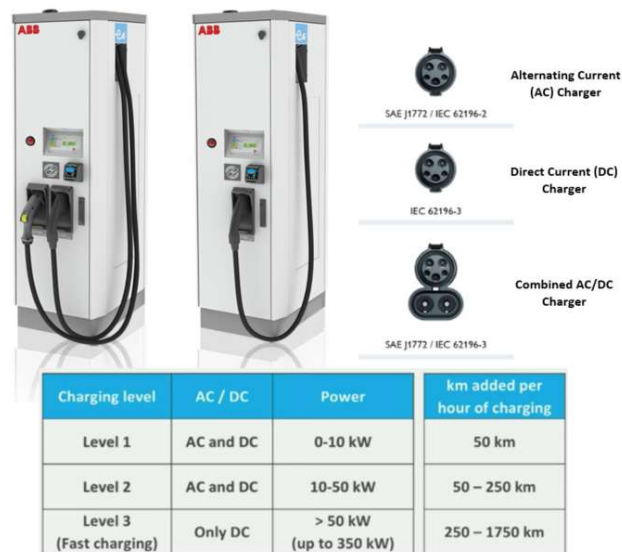
Figure 11 EV Charging Station Specs & Connector Types
