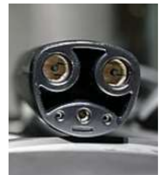
Figure 29 Tesla Supercharger North American Charge Port
